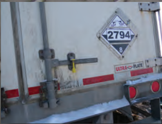
Class 8 Hazard: 50,000 lbs of Batteries
